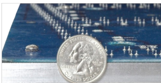
3/8" Bashplate protects LEDs
